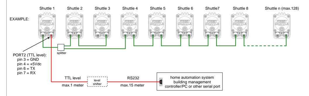
All Shuttles have the address 'OWN' and can be changed before connecting to the FX-bus. Commands are addressed directly to a Shuttle or, in some cases, globally to the entire bus. In many cases, a Shuttle responds to a command by placing a response FX message onto the bus that is picked up by the FX gateway and transmitted over the Serial Communications uplink to the Home Automation system / Controller / PC.
